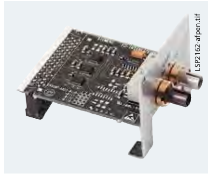
Fig. 6/20 820 nm fiber-optic communication module
