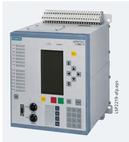
Fig. 10/5 Surface-mounting housing with screw-type terminals, example 7SA63
