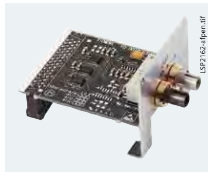
Fig. 11/14 820 nm fiber-optic communication module
