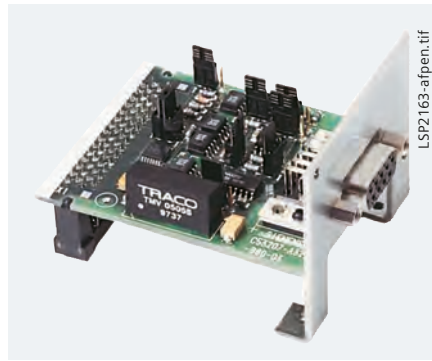
Fig. 7/51 RS232/RS485 electrical communication module
