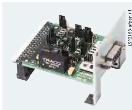
Fig. 6/22 RS232/RS485 electrical communication module
