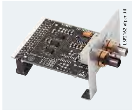
Fig. 6/62 820 nm fiber-optic communication module
